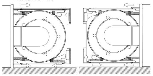
2. Drawing out a disc holder (pull return) can be easily done with inserting a propelling pencil ahead in the hole that is installed on the disc holder.
